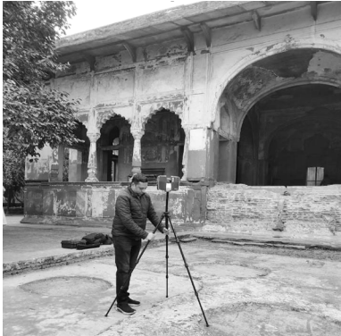
Laser scanning of Shish Mahal in progress
