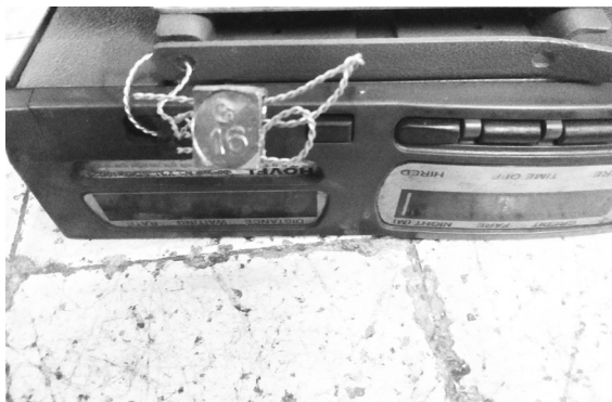
A meter sealed by the Taximeter Unit of the Department of Weights and Measures, showing the quarter (C for July-Sept) and year in which it was sealed.
